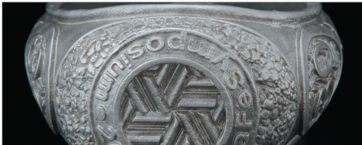
Figure 18 Cast result of a heat-cured signet ring
