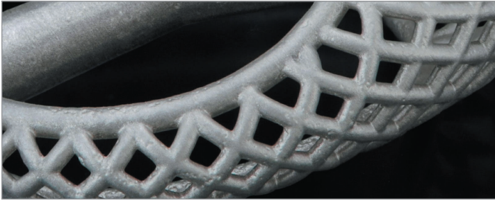
Figure 15 Cast result of a heat-cured cage ring
