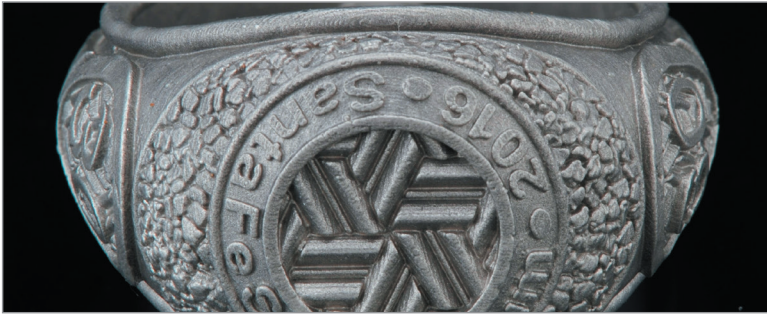
Figure 19 Cast result of a vacuum oven-cured signet ring
