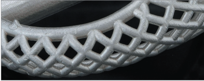
Figure 16 Cast result of a vacuum oven-cured cage ring
