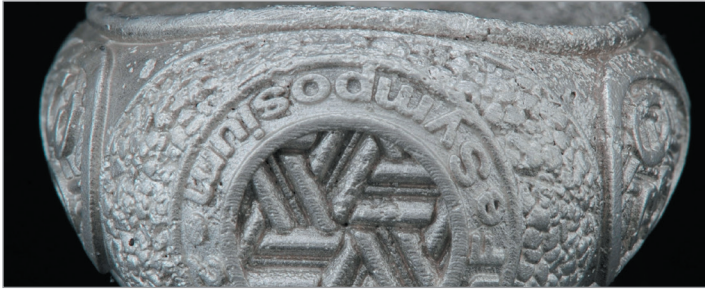
Figure 17 Cast result of a UV-cured signet ring
